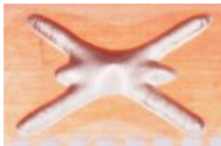
Dispense Patterns Visible solvent bleed out
