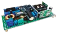
EVLSTNRG011-150 EVL011A150ADP 12 V - 150 W power supply based on TM PFC and HB LLC digital combo controller
