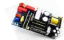
STEVAL-205GANCB 24 V - 250 W power adapter based on GaN and digital control
