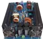
STEVAL-ISA172V2 2 kW fully digital AC-DC power supply (D-SMPS)
