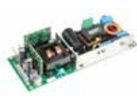
EVL011A150ADP 12 V - 150 W power supply based on TM PFC and HB LLC digital combo controller
