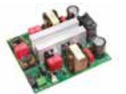
EVL4986A-1KWBL Low THD-High efficiency, 1 kW bridgeless CCM-PFC
