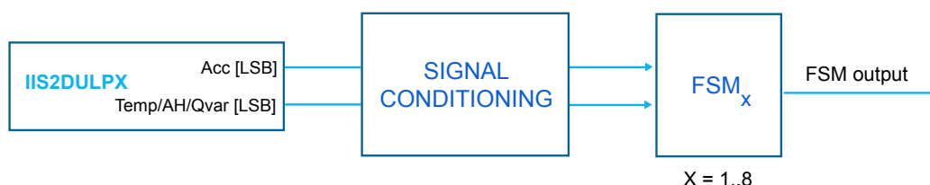
Figure 12. State machine in the IIS2DULPX
