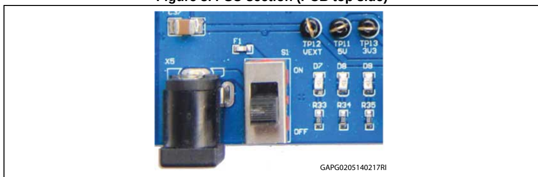
Figure 3. PSU section (PCB top side)
