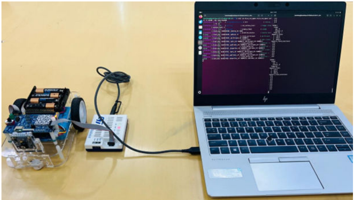
Figure 37. Micro-ROS Working Setup on STEVAL-ROBKIT1
