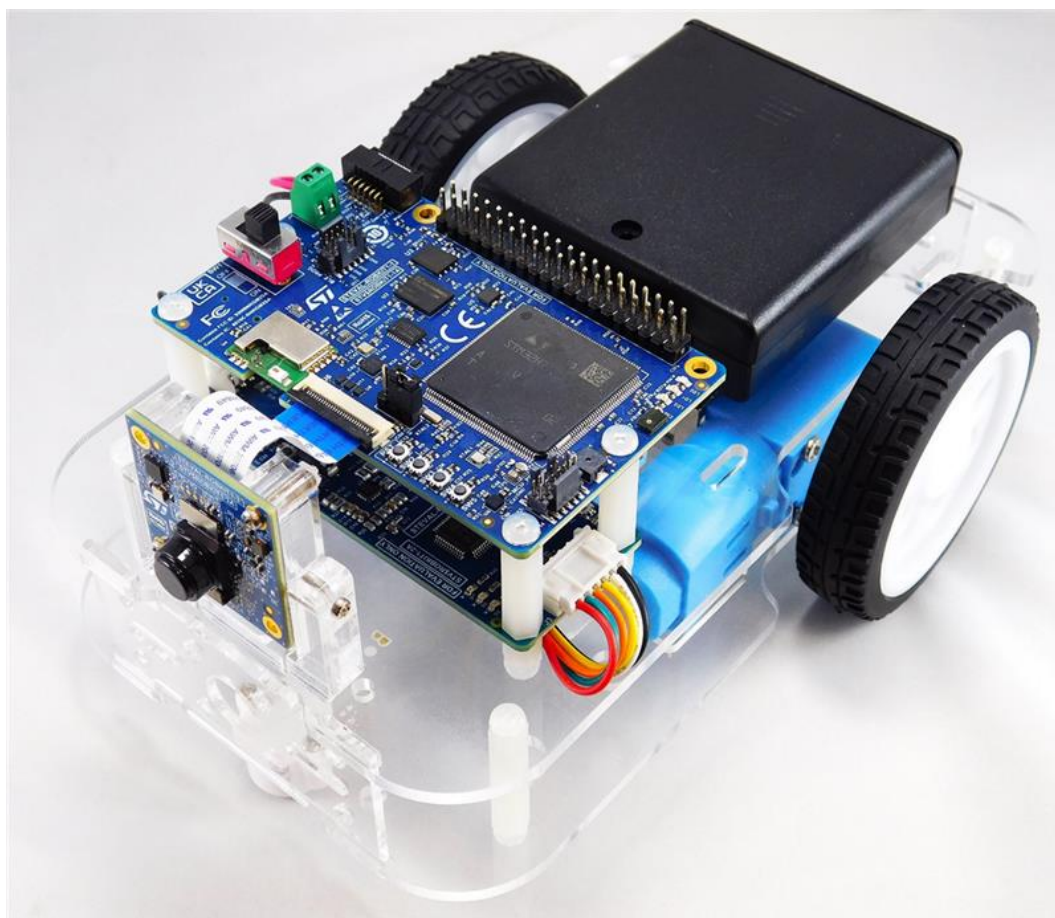
Figure 1. STEVAL-ROBKIT1 Robotic application evaluation kit
